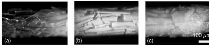
Figure 5. Optical photographs, showing three different zones in the quartz capillary, filled with microfibers M1 (thickness d = 36 \mu\text{m} ) and studied with in-situ X-ray measurements during heating. (a) Microfibers in the low-temperature zone have a transparency gradient along the crystal length with the opaque part of the crystal in the right (hot) part. (b) Opaque microfibers in the medium-temperature zone. (c) Opaque microfibers and heating products in the high-temperature zone (smaller particles). The X-ray spot size 0.5 mm was focused on this part of the capillary during the in situ X-ray study. Capillary has a diameter of 0.5 mm; wall thickness is 0.01 mm.
